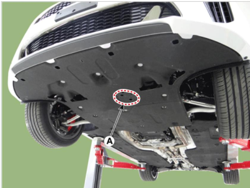
(2) Remove the oil filter cap (A).
